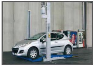
Bipark 26 is a compact double car stacker that lifts the car smoothly and quickly into position.
